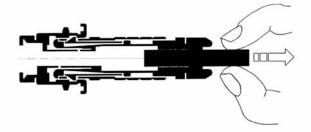
Connection cannot be broken by pulling the cable or any other parts of the plug than the outer shell.
